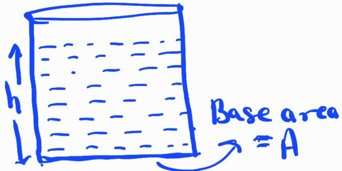
The weight of the liquid exerts the force on the bottom of the container
