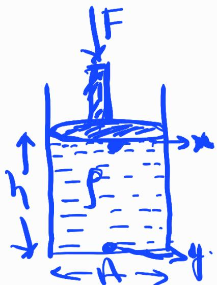
The Pressure at the Point on the fluid surface just below the Piston
