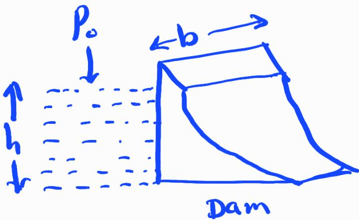
Sol: Consider the differential area of width  $dy$  and length  $b$  at a depth  $y$  from the free surface of the liquid.
